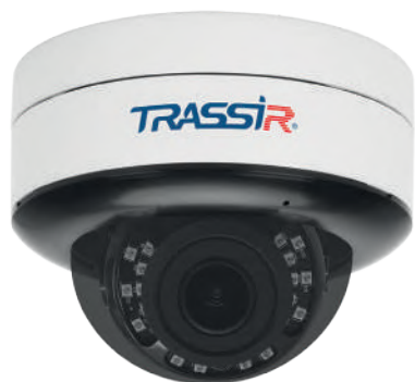
5 MP outdoor camera with varifocal lens and IR – illumination up to 25m
