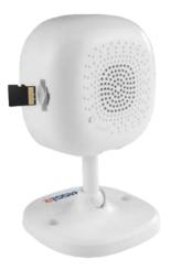
MicroSD is available for record. The camera starts the default recording to the MicroSD card when it detects motion. Use the TRASSIR Client mobile application for viewing the archive from the SD card.
